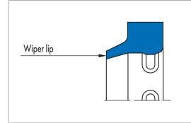
Single-acting elastomeric dirt wiper with bearing
