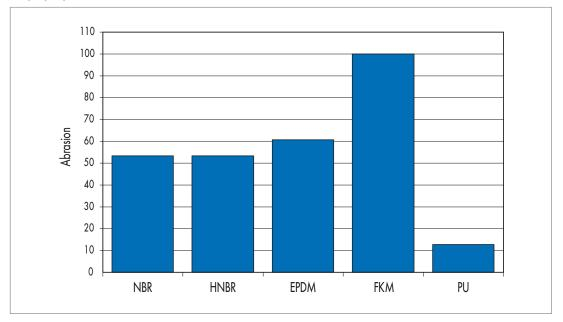
Fig. 35 Wear behaviour in comparison
