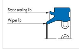
Dirt wiper with additional static sealing lip and bearing
