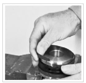
Fig. 49 Snapping in the guide back-up ring
