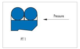
Fig. 53 Functional direction of wiper
