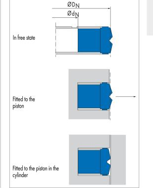
Fig. 3 Piston seal
