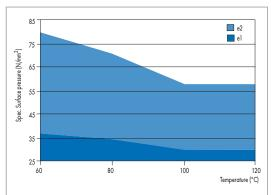
Special surface pressure for parallel load
