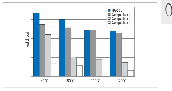
Fig. 36 Loading depending on the operating temperature
