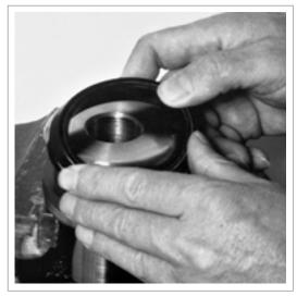
Fig. 46 Inserting sealing ring
