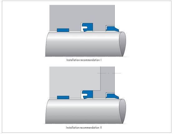
Fig. 38 Installation types of rod seals
