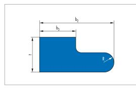
Mating rings are used for fastening and prevent axial movement of the U-rings, which can damage the sealing edges at the sealing lips. They are manufactured using extruders. The mating rings are always supplied by the metre.
