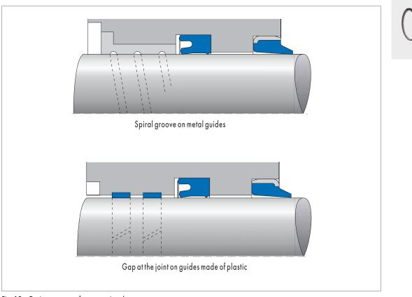
Fig. 19 Design measures for preventing drag pressure
