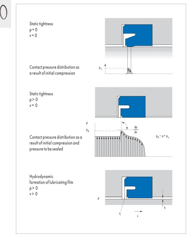
Fig. 15 Compression curve and hydrodynamic lubrication film formation
