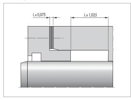
Adjustable housings have the advantage of an optimal adjustment option for the sealing effect with minimal idling friction. After a lengthy period of running and incipient wear on the seal tightening the gland can extend the durability and significantly delay a system standstill. For adjustable housings an extension of 2,5% and an adjustability of 7,5% of dimension L is recommended. Non-adjustable housings have the advantage
