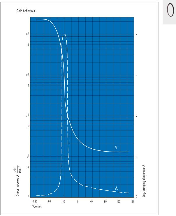
Fig. 20 Graph: torsion vibration test in accordance with DIN 53445; dynamic shear modulus G and logarithmic decrement  $\Lambda$  of a Simrit material based on CR
