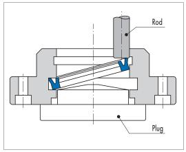
Fig. 41 Installation aid for rod seals
