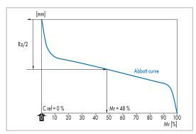
Fig. 30 Simrit material component definition
