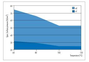
Special surface pressure for parallel load
