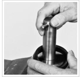
Fig. 47 Inserting mounting pin
