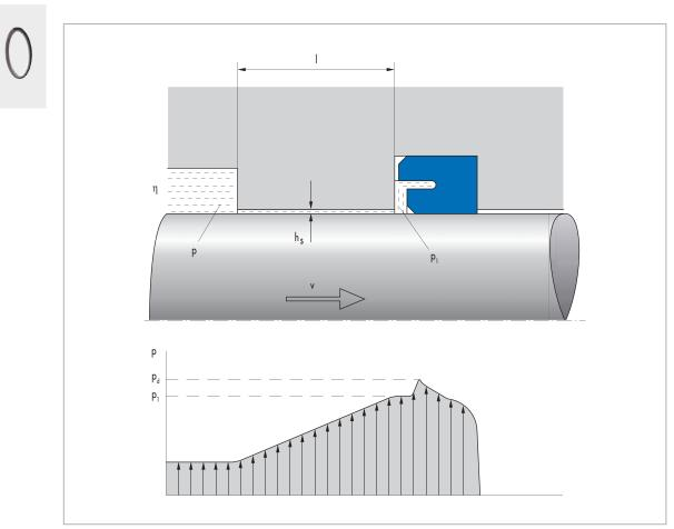
Fig. 17 Hydrodynamic drag pressure
