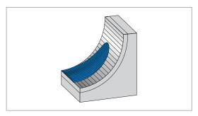
Fig. 9 Guide ring with convex profiling
