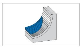
Fig. 8 Guide ring of fabric-base laminate
