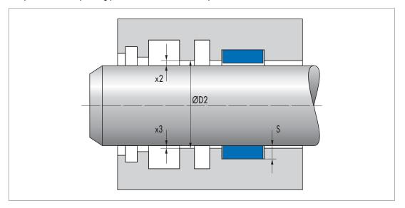
Fig. 14 Sealing gap
