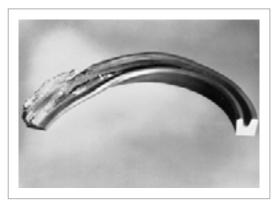
Fig. 18 U-ring destroyed by hydrodynamic pressure build-up
