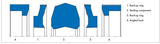
Fig. 52 Fitting of Merkel Compact Seal L 43
