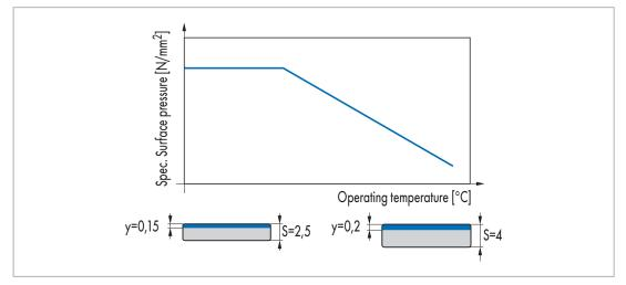
Fig. 13 Deflection at maximum surface pressure
