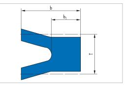
U-rings are produced, extruded and bonded to the butt for use as piston or rod seals. U-rings made of NBR and FKM are also available with vulcanisation to butt. They can be supplied at extremely short notice.
