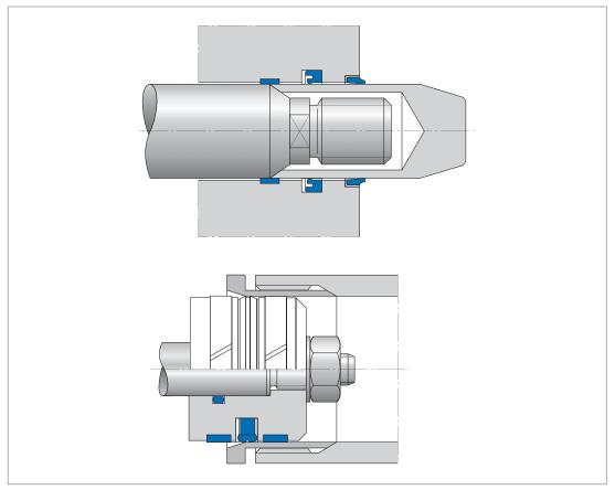
Fig. 37 Covering threads when mounting seals
