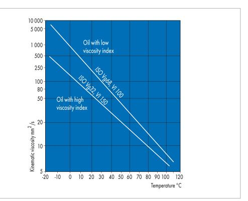
Fig. 21 Viscosity-temperature behaviour of various hydraulic oils
