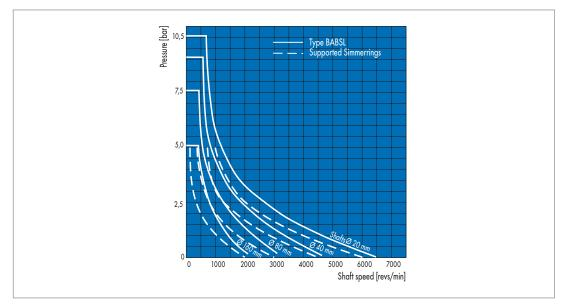
Permissible pressure in the unit for Simmerrings (type BABSL), as well as for Simmerrings with back-up rings.
