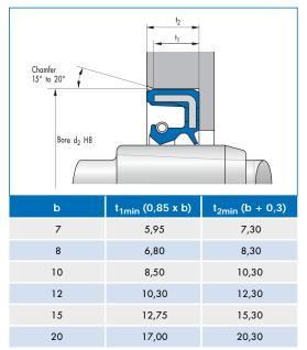
Fig. 35 Depth and chamfer on the locating bore
