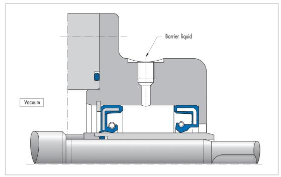
Fig. 7 Sealing against a vacuum
