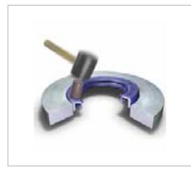
Fig. 47 Inclined fitting not permissible WRONG!
