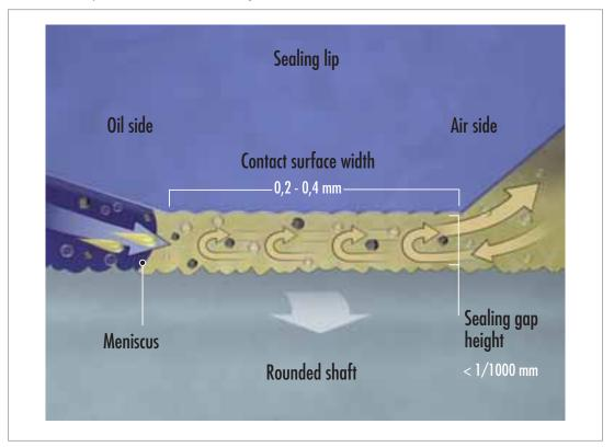
Fig. 13 Micro-pumping action of sealing lip in the shaft-sealing lip contact zone
