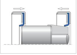
Fig. 51 Fitting a Simmerring with sealing lip made of PTFE
