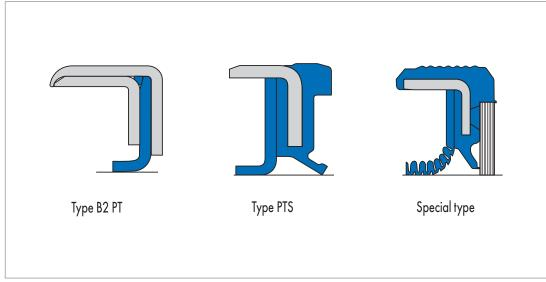
Fig. 36 Simmerrings with PTFE sealing lip
