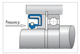
Fig. 26 Installation of a Simmerring with back-up ring
