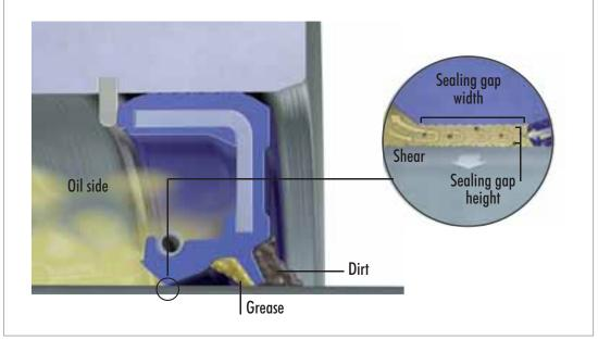
Fig. 10 Simmerring<sup>®</sup> seal-shaft contact area
