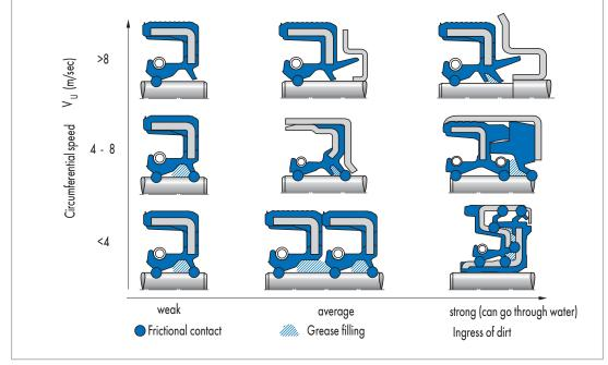
Fig. 27 Simmerrings for secure sealing against dirt
