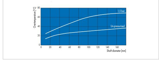
Fig. 23 Overtemperature at the sealing edge of a Simmerring with un-pressurised sealing and with application of pressure, Engine oil: SAE 20, rotational speed: 3000 U/min, oil level: centre of shaft
