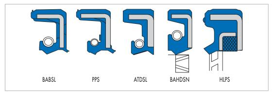
Fig. 24 Types for Simmerrings which can be pressurised
