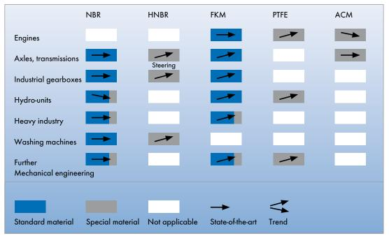
Fig. 19 Materials applications for Simmerrings
