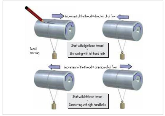
Fig. 30 Determining lead on the shaft
