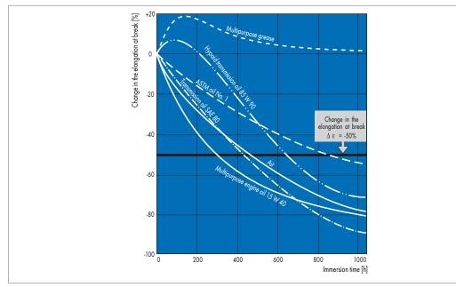
Fig. 17 Change in the elongation at break of NBR on immersion at 100 °C in various media
