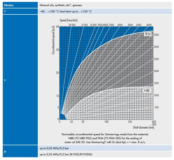
\* With synthetic oils (polyalkylene glycols/polyalphaolefins) it is to be noted that the maximum operating temperature of 80 °C must not be exceeded.
