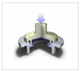
Fig. 46 Fitting "back abutment face to front". Outside diameter of the pilot shaft approx. 0,5 mm smaller than the inner lining diameter of the seal. Please enquire if necessary.
