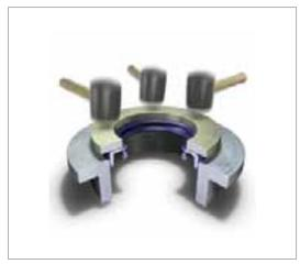
Fig. 49 Permissible hammer assembly USE MOUNTING PLATE!
