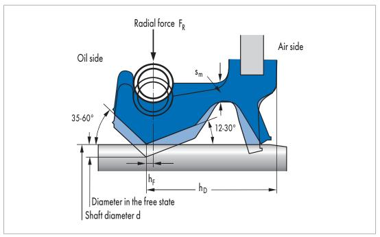
Fig. 11 Dimensions of the sealing lip profile
