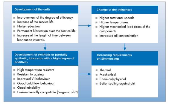
Fig. 18 Increasing requirements on Simmerrings
