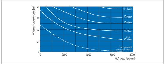
Fig. 33 Deviation of coaxiality and of runout as a function of rotational speed for Type BABSL
