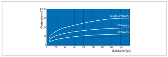
Fig. 22 Overtemperature at the sealing edge of a Simmerring as a function of the rotational speed Engine oil SAE 20, oil bath temperature 100 °C, oil level: centre of shaft
