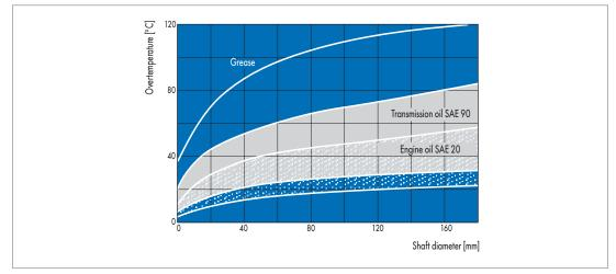
Fig. 21 Overtemperature at the sealing edge of a Simmerring when sealing differing media, temperature of oil bath 100 °C, rotational speed 3000 rpm
