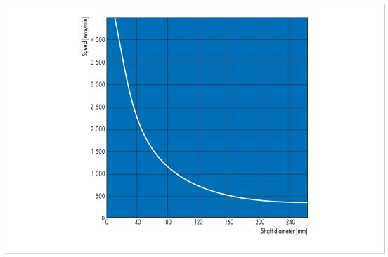
Fig. 28 Permissible rotational speeds with rotating Simmerrings on fixed shafts If limits are exceeded, please consult us!
