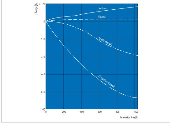
Fig. 16 Changes of the characteristic values of an NBR material as a function of storage time; immersed in gearbox oil SAE 80 at 100 °C
