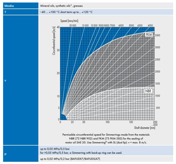
\* With synthetic oils (polyalkylene glycols/polyalphaolefins) it is to be noted that the maximum operating temperature of 80 °C must not be exceeded.
