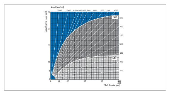
Permissible circumferential speed for Simmerrings made of the material NBR (72 NBR 902) and FKM (75 FKM 585) when sealing engine oil SAE 20. Usage of Simmerring with SL (dust lip): v = max. 8 m/s.
