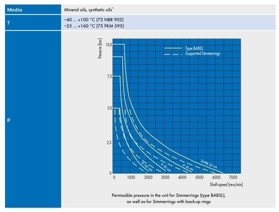
\* With synthetic oils (polyalkylene glycols/polyalphaolefins) it is to be noted that the maximum operating temperature of 80 °C must not be exceeded (only for use of NBR).
