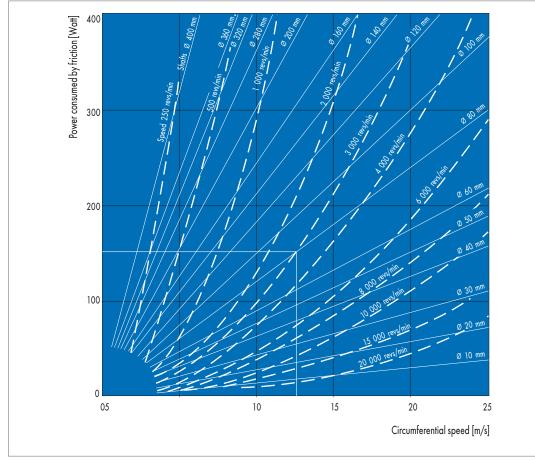
Fig. 15 Recommended values for the friction loss on a Simmerring in engine oil SAE 20, at T=100 °C, Example: shaft ∅ d1=80 mm, speed n=3000 U/min, friction loss approx. 150 W
