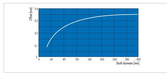
Fig. 31 Max. deviation of the concentricity as a function of the shaft diameter
