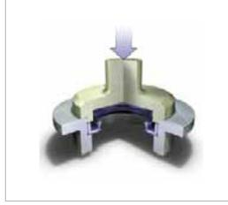
Fig. 45 Fitting with hydraulic or pneumatic assembly press. Diameter of metal tool face 5 mm to 10 mm larger than seal outside diameter (d<sub>2</sub>)
